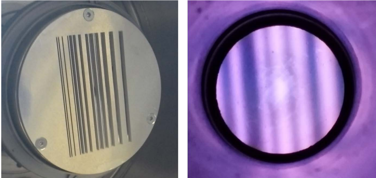
Figure 1 – a) Photograph of patterned Electrode A composed of 13 slits with different widths and spacings. The slits are 60 mm long. b) Photo taken through a transparent substrate showing ignition of plasma within slits of electrode.
